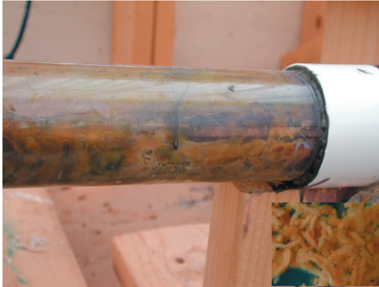
Closeup of the clear outflow pipe demonstrating the biofouling activity that is occurring in the bench scale model. The insert is a photo of the microscopic floc caused by iron bacteria in water systems that result in clogging of drains and wells.
