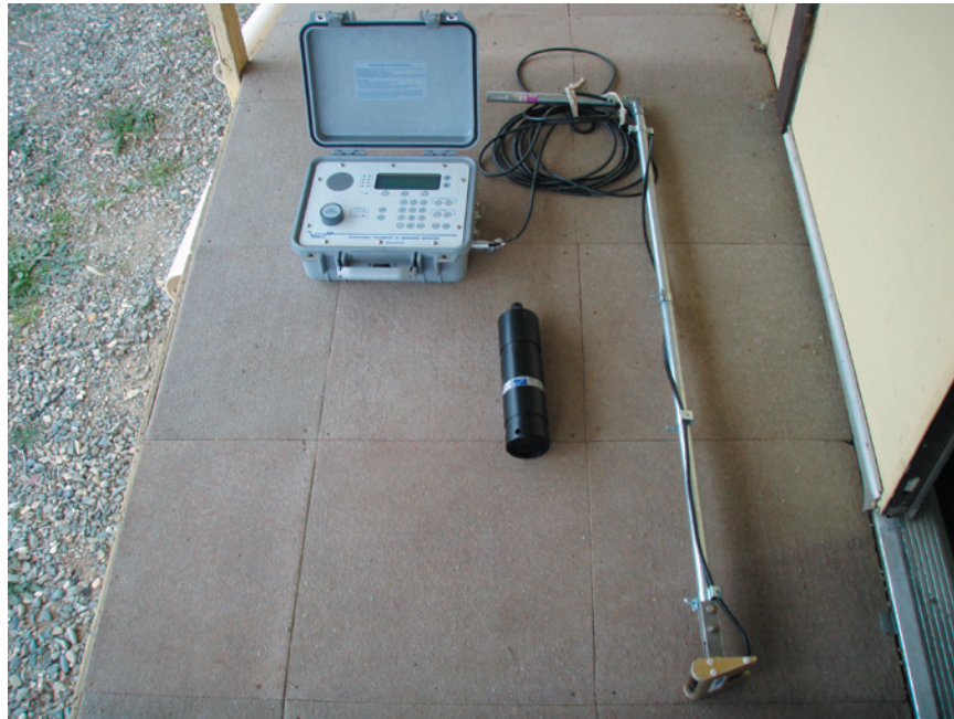
A portable receiver with a directional hydrophone detects hydroacoustically tagged green sturgeon.
