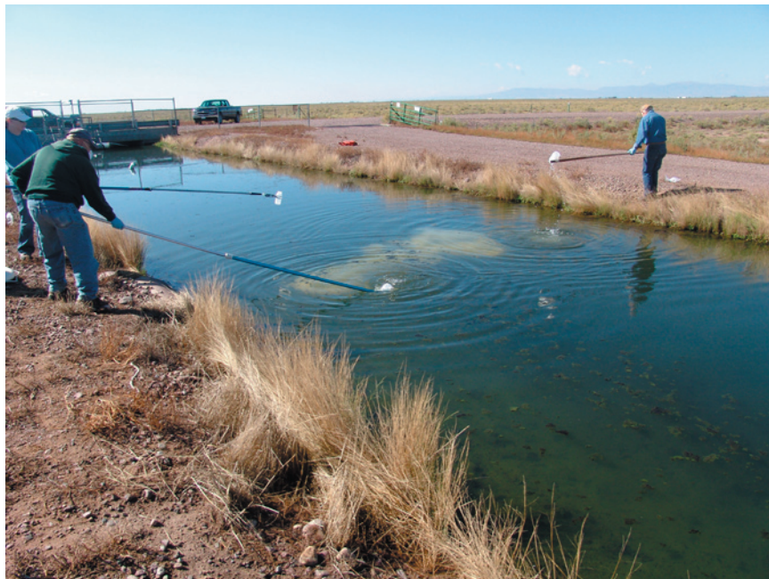
PAK27 being applied to the Franklin Eddy Canal to determine the effect on the canal's TDS concentration over a 300-foot long test section. Once applied, the formulation started to release the active ingredient resulting in a white cloud that spread from the initial application site. Water samples were then collected at upstream and downstream sampling sites to determine TDS concentrations.
