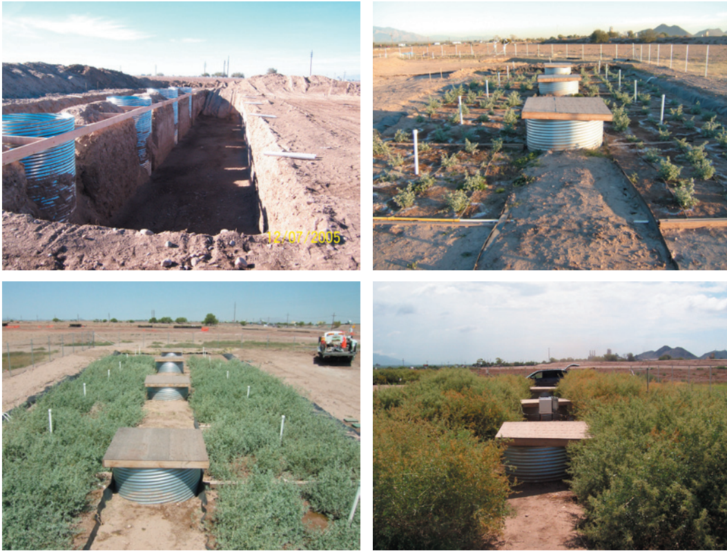
Photographs of lined Atriplex plot development over time (left top). The plots were fitted with an irrigation system and Atriplex were transplanted. Plant growth over the course of the next year was documented by photography, December 2006 (right top), April 2007 (left bottom) and September 2007 (right bottom).
