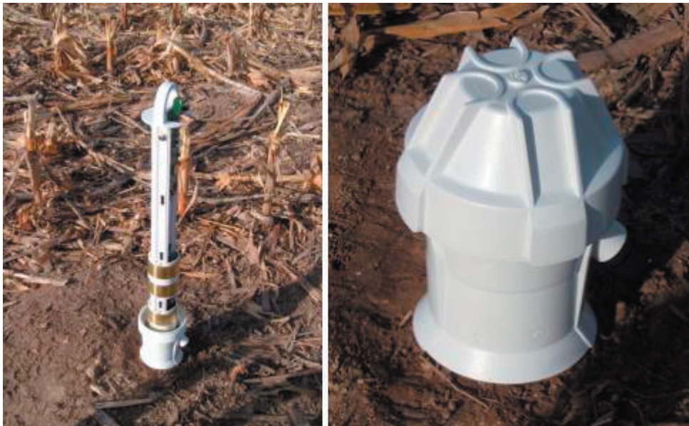
An EnviroSMART probe installed in a terrace channel used to measure volumetric water content at six depths up to 6 feet. The picture at the left shows the probe installation into the access tube, and the picture at the right shows the completed installation.
