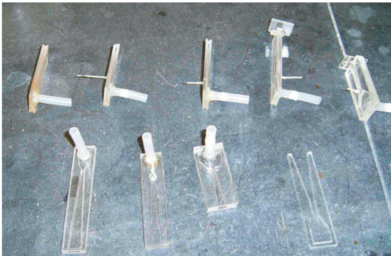
Other examples of venturi nozzles.
