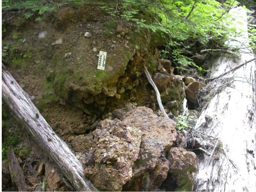
Photo 5. The majority of the Sidney mine waste dump comprises ferricrete which forms when waste material has been cemented with iron oxides into rock, view to the southeast (photo by G. Graham, 8/3/2006).
