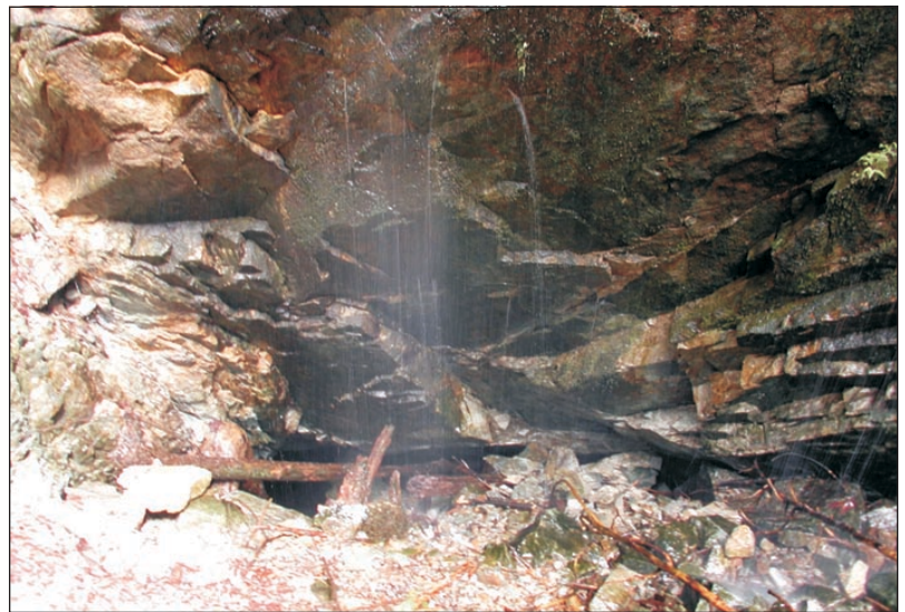
Figure 6. A 4 x 4 foot opening above stope 3. The log is approximately 1 foot in diameter.
