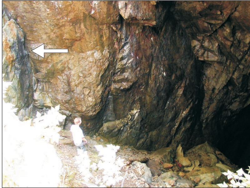
Figure 10. Entrance to stope 11. Note the mineralized vein on the wall on the left side of the photo (arrow). View is to the northeast.
