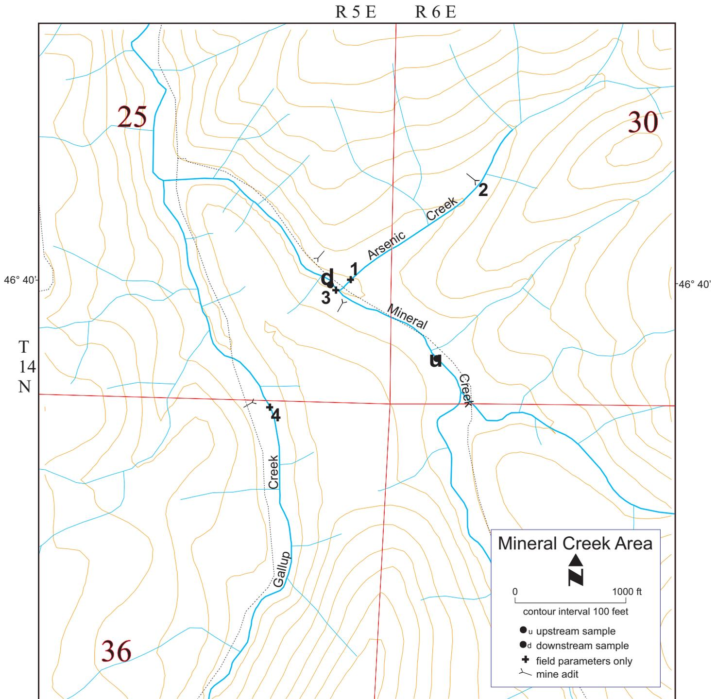
**Figure 10. Location of Water and Sediment Samples Collected in Mineral Creek, Mineral Creek Area**
