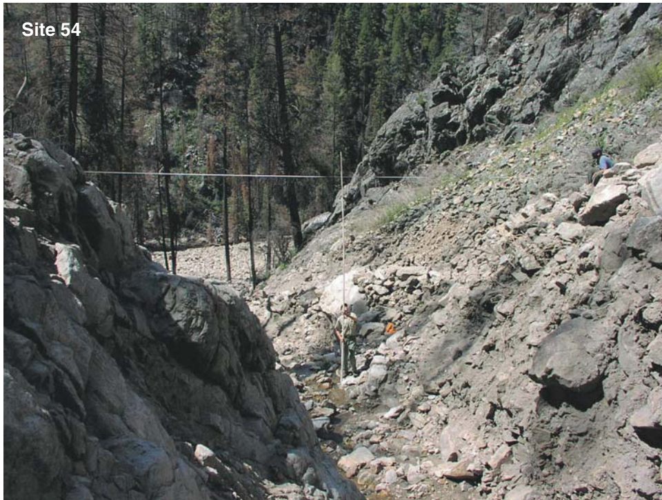
Figure 8. Measuring debris-flow channel section at two unnamed tributaries to Sleeping Child Creek (sites 53 and 54), Montana.
