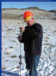
Above left: Dr. Klusman extracts a 1 meter soil gas sample.
