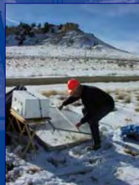
Above left: Dr. Klusman extracts a 1 meter soil gas sample.
