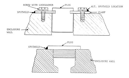
WELD (OR BRAZE) MAY BE ON PLUG, CLAMP, OR FASTENING
