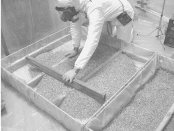
Figure 13: Evenly Distributing the Vermiculite Attic Insulation in the Simulated Attic Trusses
