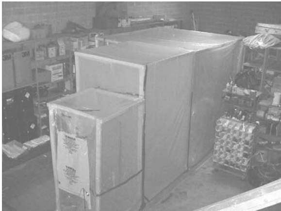
Figure 9: Overhead View of Containment System Used for Simulation of Consumer Use of Vermiculite Attic Insulation
