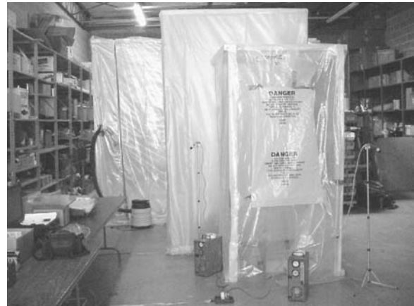
Figure 10: Front View of Containment System Used for Simulation of Residential Use of Vermiculite Attic Insulation
