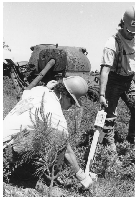
Contractors search for buried unexploded ordnance in the impact area at Camp Edwards on Cape Cod using a magnometer device.
