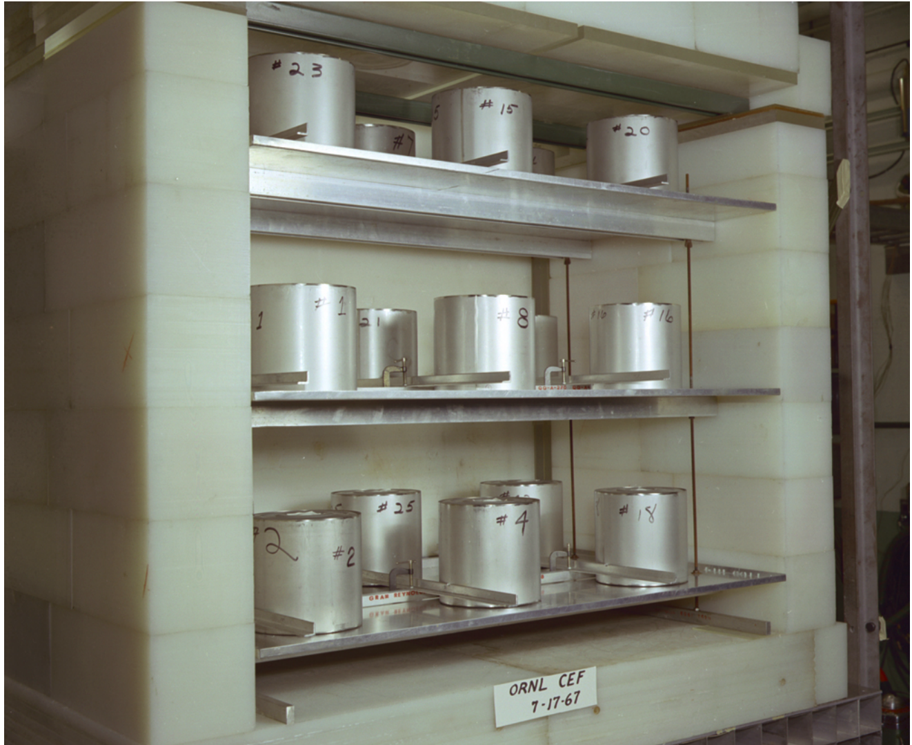
Figure 4. Photograph of the fixed table during Experiment 85, a polyethylene reflected 27-cylinder array.
