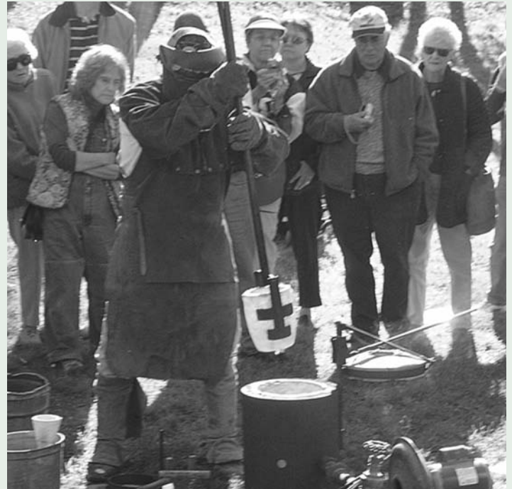
Glen Campbell, owner of an artist foundry in West Rutland, Vermont, uses a portable furnace to cast two bronze sculptures using the ancient “lost wax” bronze casting method. This is the same method used by Augustus Saint-Gaudens to cast everything from his detailed portrait reliefs to huge monuments such as the Shaw Memorial. Casting demonstrations like this are rarely seen by the general public. Fritz Maslan of Cornish is one of the artists that had his sculpture cast in bronze during the demonstration.
