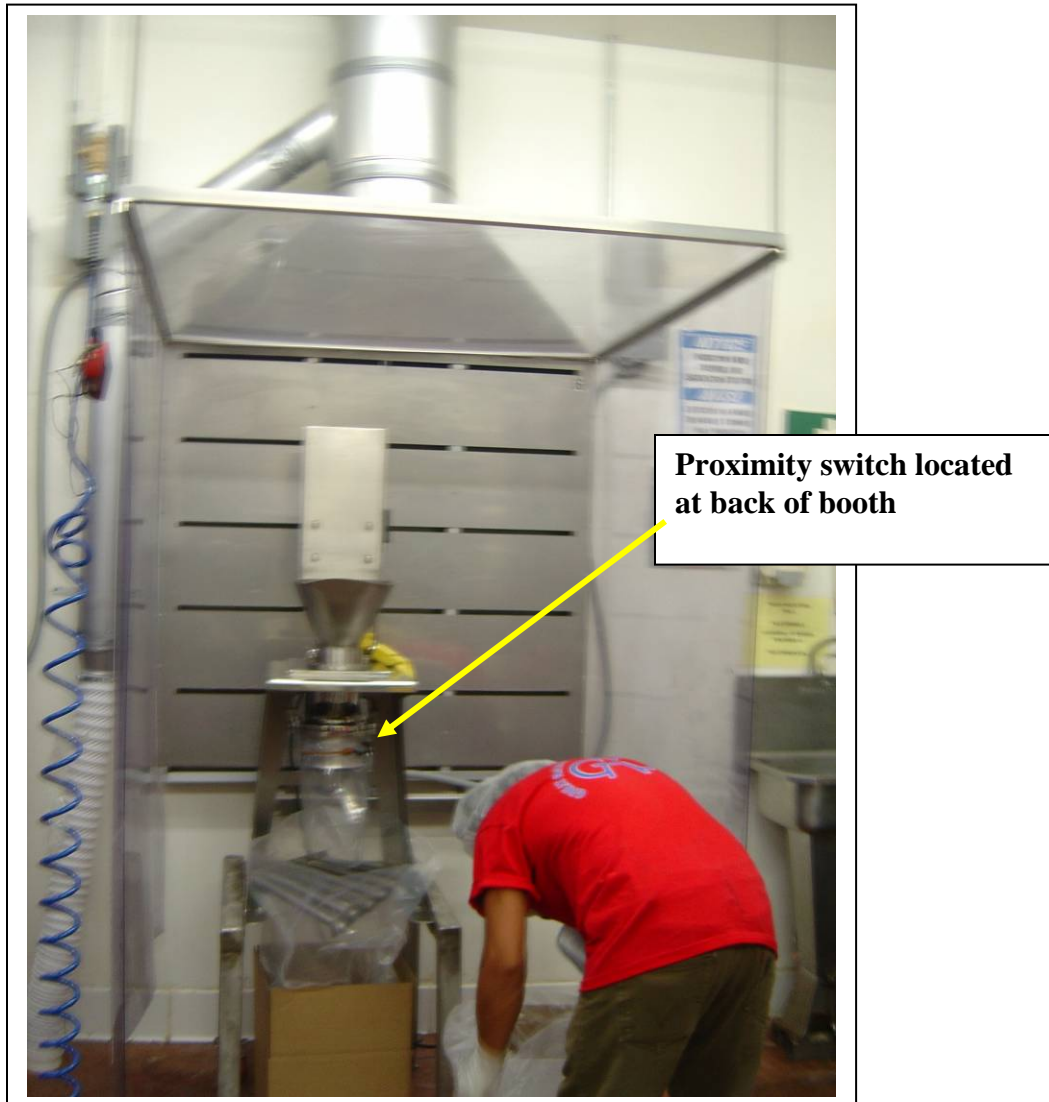
Figure 9. Packaging of butter flavored powder in the ventilated mixing tank booth
