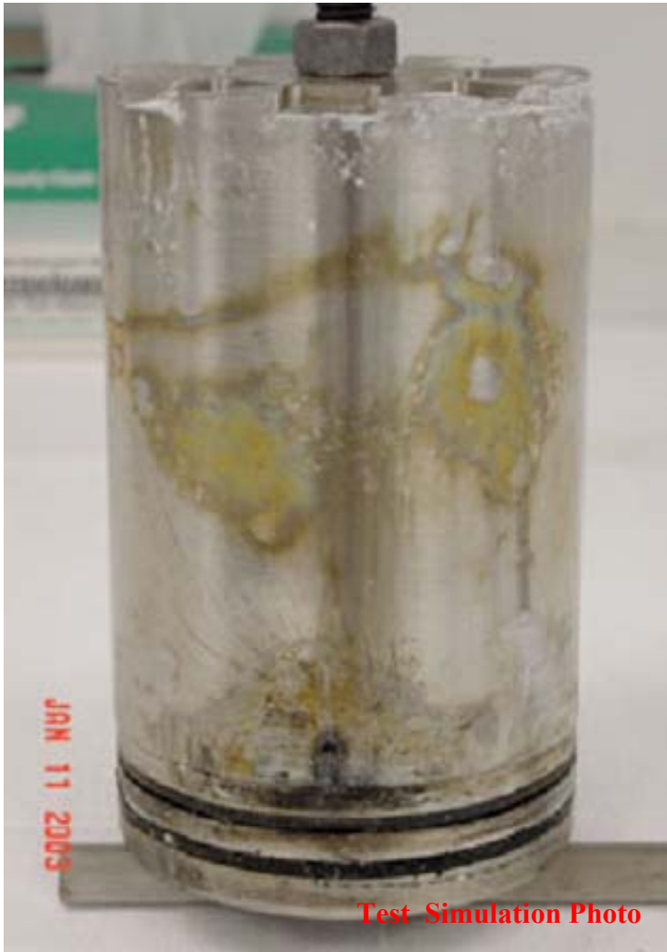
Test #4 (leak rate: 0.0012 gpm) Nozzle outer diameter showing buildup of white deposits at discharge of annulus
