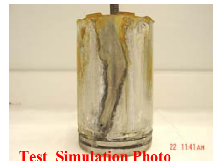
Test #5 (leak rate: 0.0006 gpm) Crusty yellow deposit buildup on nozzle wall at annulus discharge
