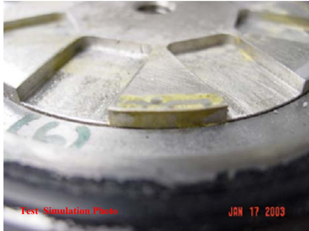
Test #5 (leak rate: 0.0006 gpm) Crusty yellow deposit buildup on nozzle wall at annulus discharge
