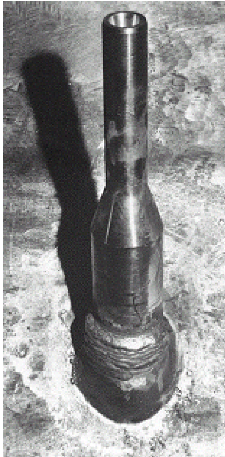
Modified IMI nozzle (inside of reactor vessel)
