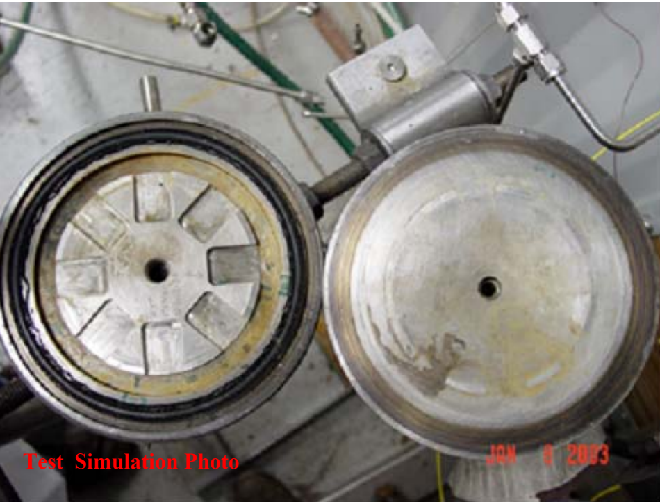
Test #3 (leak rate: 0.0004 gpm) Post test view of nozzle/head assembly & thrust plate
