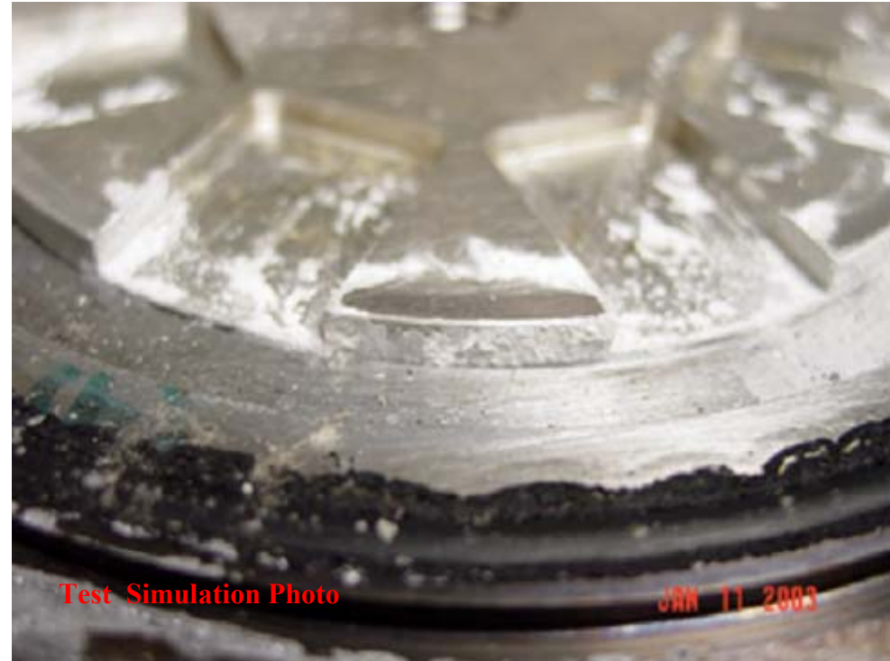
Test #4 (leak rate: 0.0012 gpm) Close-up of head-to-nozzle annulus showing buildup of white deposit at exit of annulus
