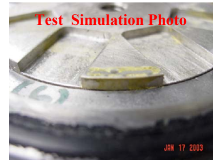
Test #5 (leak rate: 0.0006 gpm) Crusty yellow deposit buildup on nozzle wall at annulus discharge
