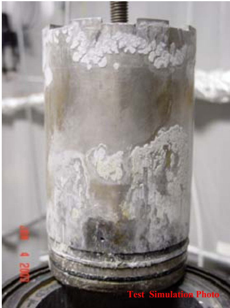
Test #2 (leak rate: 0.0017 gpm) Nozzle OD showing buildup of white deposits
