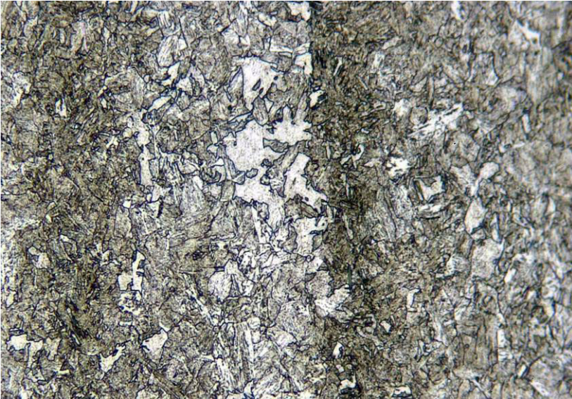
Procured Canceled Plant Material for Current MRP BAC Testing Program Bainitic Microstructure
