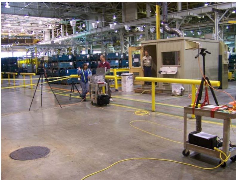
Figure 5-5: Photograph looking the other way in the same corridor of the stamping plant. The high-frequency directional antennas are shown. The photograph shows the VNA and the optical fiber linking the transmitting and receiving antennas.
