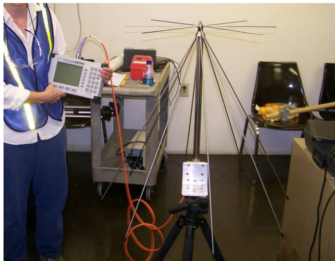
Figure 4-2: Photograph of the portable spectrum analyzer and omnidirectional antenna used to collect snapshots of spectrum throughout the three plants. The antennas shown here were used at frequencies up to 1 GHz. Other omnidirectional antennas were used at higher frequencies.
