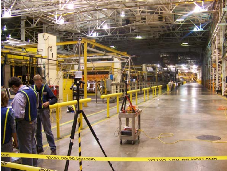
Figure 5-4: Photograph of the long corridor in the stamping plant where the UWB scattering measurements were made. The low-frequency omnidirectional antennas are shown. The VNA is located near the NIST staff at the left side of the photo.
