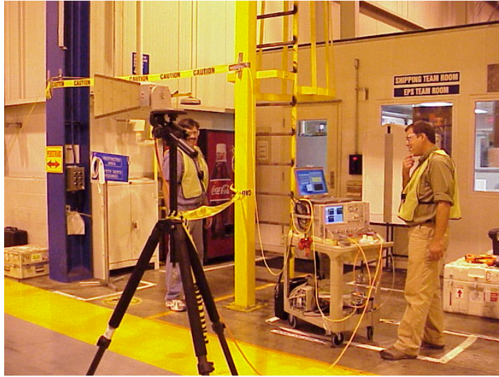
Figure 5-8: VNA set-up in the engine plant. The directional transmit antenna is shown in the foreground. The corridor shown in Figure 5-7 continues to the left side of this picture.
