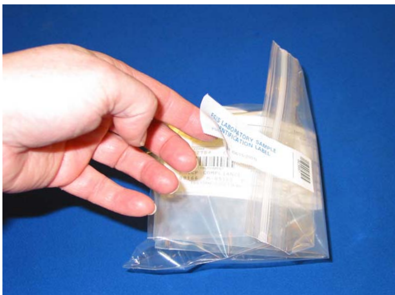
Figure 4 – Placement of the bar-coded Identification Label on the zipper lock bag containing the sample and submission form.
