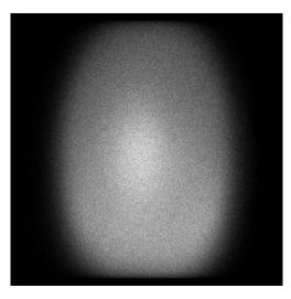
Intensity, I(x, y), is proportional to the estimated likelihood that a minutiae will be found by a template generator at (x,y).
