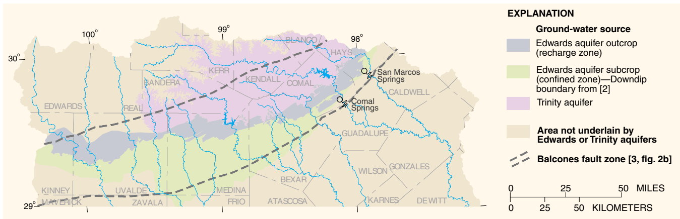
Figure 2. Areal extent of the Edwards and Trinity aquifers sampled during 1996–98 (modified from [4]). The outcrop of the Edwards aquifer essentially is the recharge zone; the subcrop essentially is the confined zone. The outcrop of the Trinity aquifer is approximately coincident with the Hill Country. The subcrop of the Trinity aquifer (not shown), which extends beneath the Edwards aquifer, is not a source of water supply in the region and was not sampled.
