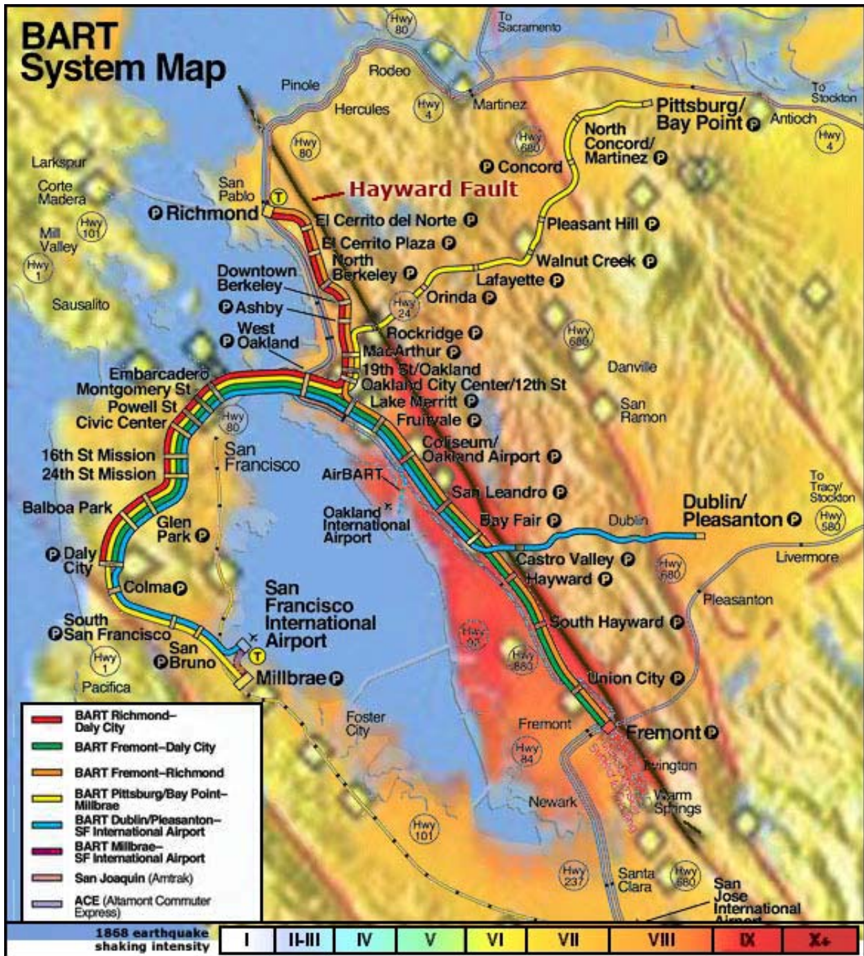
Figure 4. 1868 Hayward Earthquake Shaking Intensity Map with the BART System. The map of the San Francisco Bay Region shows the location of the BART rail system, the location of the Hayward Fault, and the earthquake shaking intensity from the USGS 1868 Hayward earthquake shakemap. The BART system is a useful indicator of the intensely urbanized corridor of the East Bay region relative to the location of the fault. For more information about the 1868 Hayward earthquake and its shakemap, see USGS Earthquake Hazards Program, 2007.
