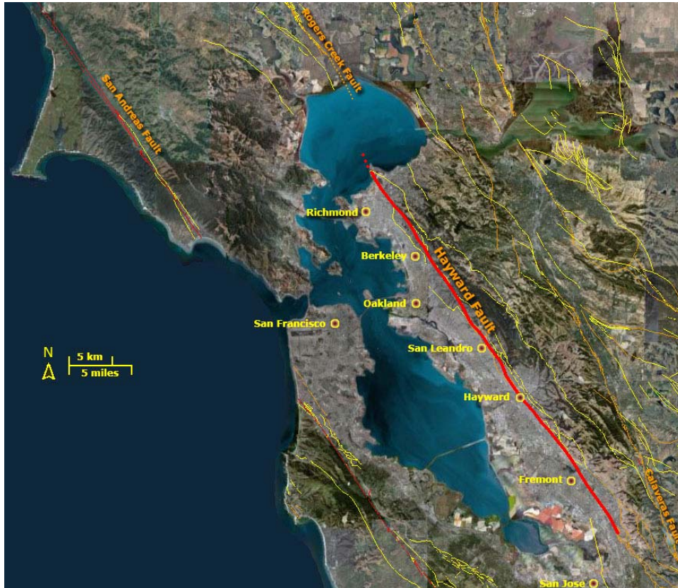
Figure 2. Location of the Hayward Fault. Fault systems in the San Francisco Bay region are shown on a satellite composite image modified from Google Earth. Faults that have had major earthquakes in historic times (since 1776) are shown in red. Faults that display movement or earthquake history in roughly the last 10,000 years (Holocene Epoch) are shown in orange. Older faults that display evidence of having activity in the last 2 million years (Quaternary Period) are shown in yellow. Fault data from Graymer and others (2006).
