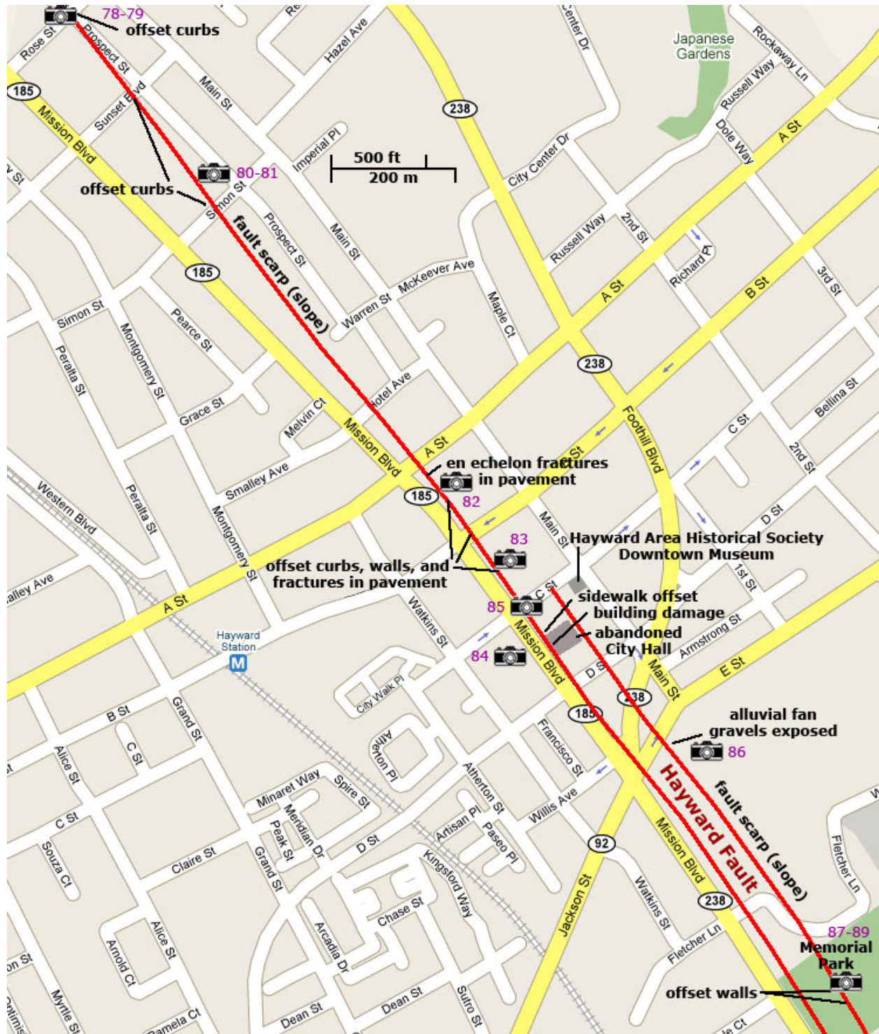
Figure 77. Map showing the Hayward Fault in the downtown Hayward area. Purple numbers designate photograph locations.
