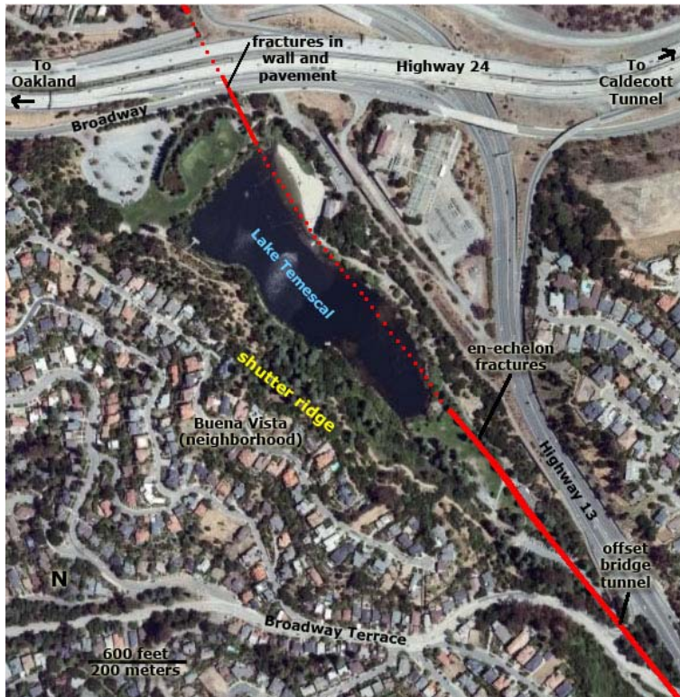
Figure 38. A Google Earth image map showing the location of the Hayward Fault and associated features in the Lake Temescal area. The Buena Vista neighborhood is on the shutteridge on the west side of the fault at Lake Tamescal. Highway 13 runs south from the intersection of Highway 24 down the rift valley of the Hayward Fault for much of its route. Temescal Lake was built during 1866 and 1869 by damming Temescal Creek, which happens to be offset more than 1.5 miles (2 km) right-laterally by the fault. The ridge to the west blocks the outflow of the creek, but the blockage is caused by the large displacement and the slowing of the stream by the reduced gradient along the fault, and probably not by "sagging".
