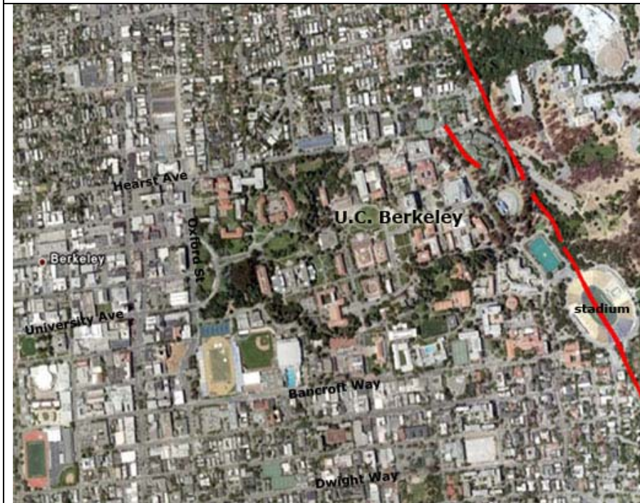
Figure 119. The Berkeley area is one of the most urbanized landscapes in the East Bay. This satellite view shows that the California Memorial Stadium next to the University of California, Berkeley, is bisected by the Hayward Fault in the northeast corner of the image.
