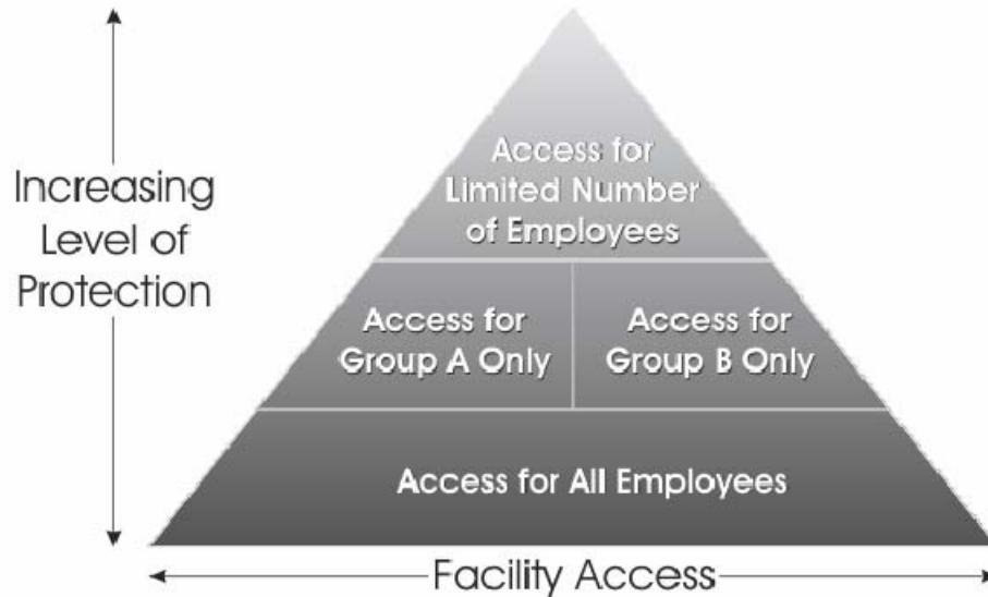
Figure 2. Example of varying employee access levels by sensitivity of the operation. Areas containing the most vulnerable operations should be restricted to a limited number of employees, and these employees should receive background investigations and additional training.
