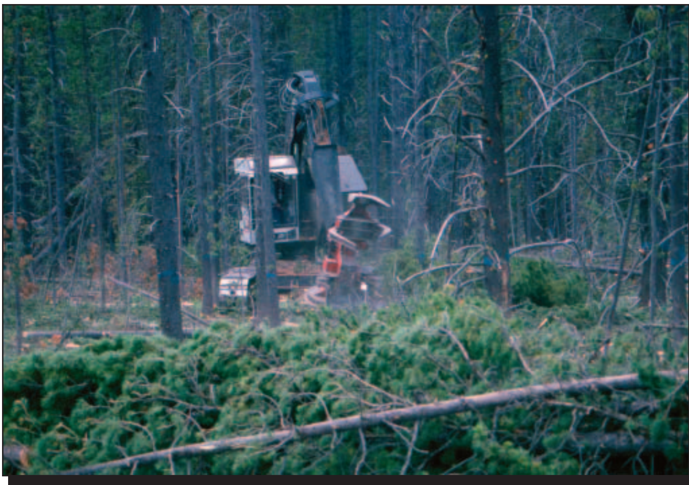
Figure 4—Mechanical harvests can successfully remove smaller biomass material while leaving larger trees.
