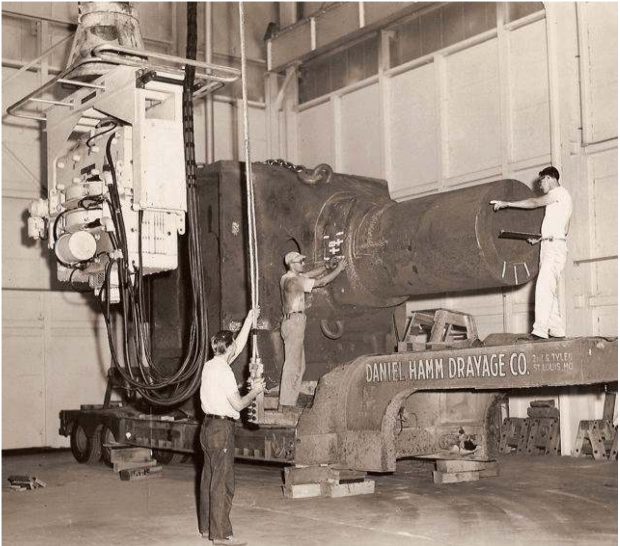
Figure 19. Betatron Radiography of the Axle of a Power Shovel Cast at GSI
