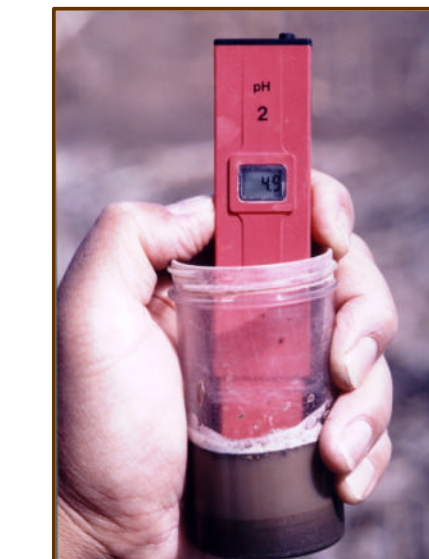
Soil pH can be measured with a pocket pH meter.
