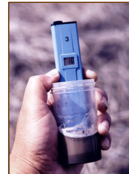
A pocket electrical conductivity meter is a quick method to measure salts in the soil solution.
