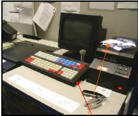
Mail handlers employed long reaches to place packages on a scale; computer and keyboard were non-adjustable and placed to side causing workers to twist their torsos to talk to customers.
