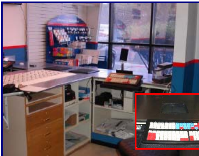
Counter height and adjustable computer keyboard allow work in neutral position; keyboard is directly in front of worker eliminating twisting of the worker's torso.
