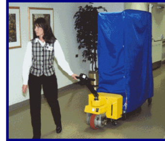
Automated tugging device reduces risk of back injury.
