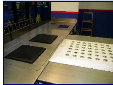
Workers can slide parcels from scales across a conveyor surface and onto a scissors lift table without manual lifting.
