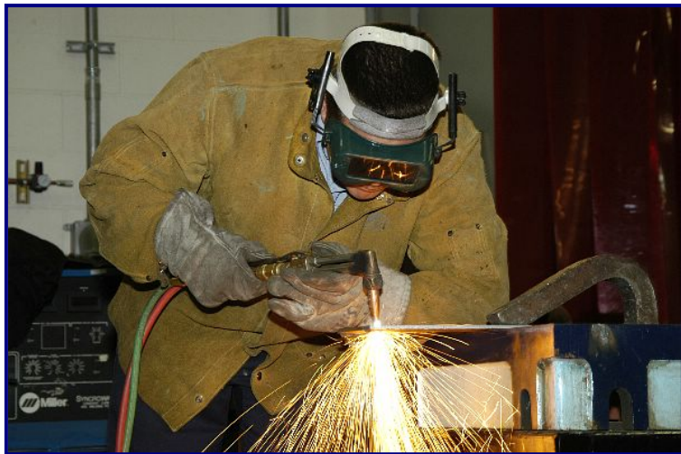
Hull Maintenance Technician 3rd Class shapes parts out of metal with a cutting torch at the Puget Sound Intermediate Maintenance Facility.
