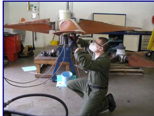
Prior to introduction of the propeller fixture, a Sailor is shown kneeling beneath a propeller and reaching overhead. Prolonged work in such postures can increase the likelihood of WMSDs
