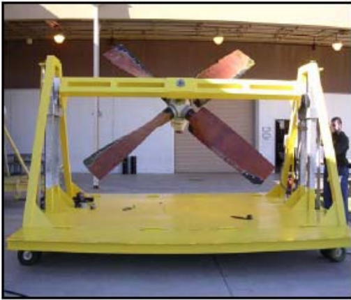
A 900 pound propeller is transported on a lightweight fixture to the Propeller Shop for repair and maintenance.
