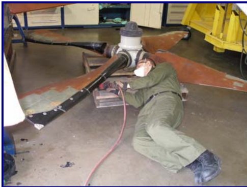
Prior to ergonomic intervention, Sailors had to assume awkward postures to work on a propeller.
