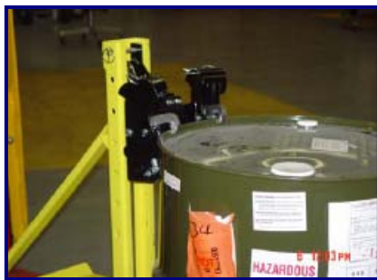
Top hook of drum handler securely grasps drum frame
