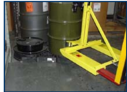
Stabilizer secures drum in upright position
