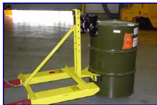
Drum handler attached to forklift eliminates manual lifting of heavy drums.
