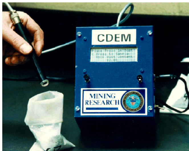
Figure 1.—The CDEM is used to analyze the composition of a coal and rock dust mixture.
