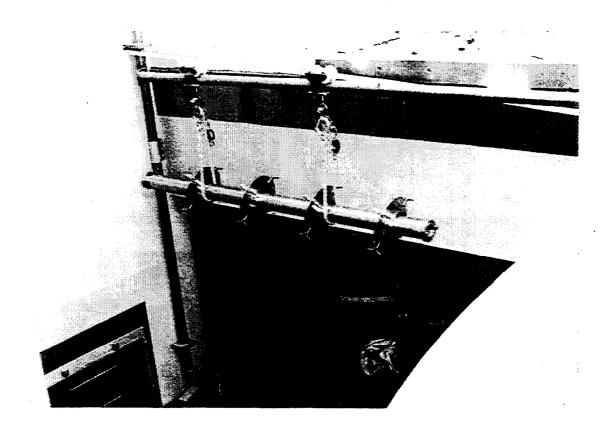
Figure 6: The intensifier bar for a PK-150 cubic foot blender shown in its storage position.
