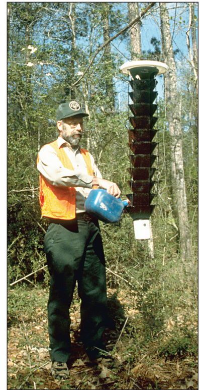
Figure 2. Lindgren funnel trap.
