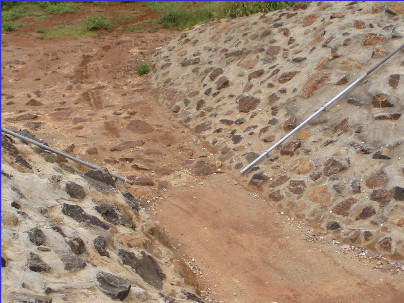
Typical Crest-Gage Mounting
