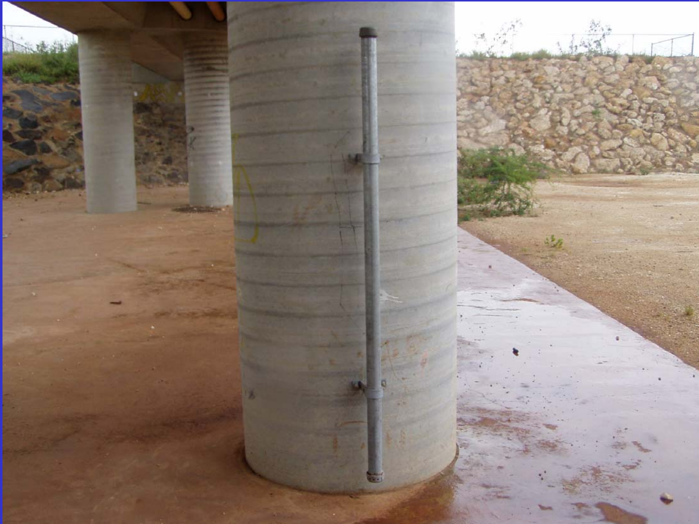
Typical Crest-Gage Mounting
