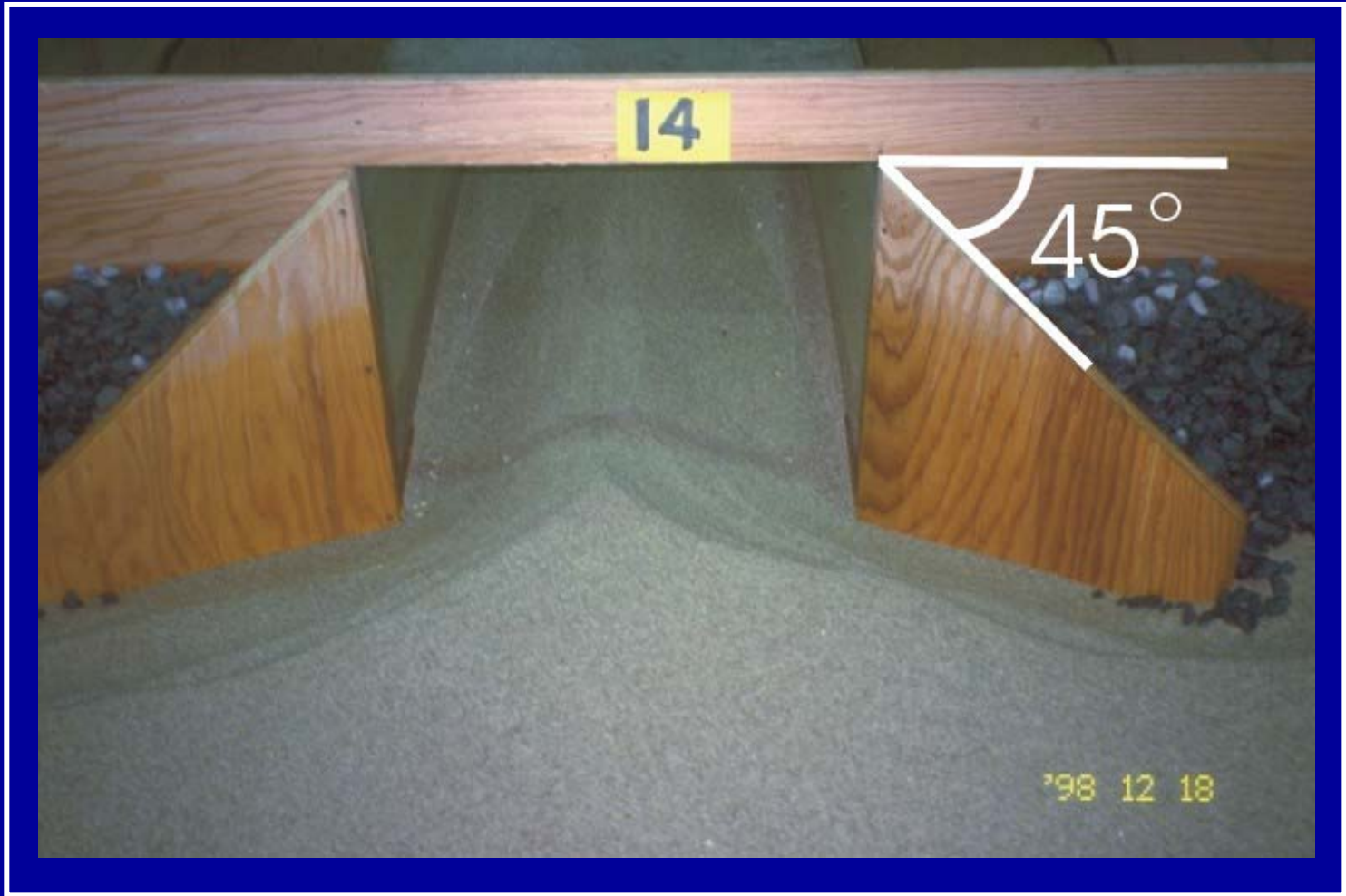
rectangular model with wingwalls
