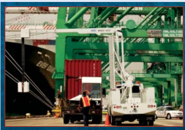
U.S. Customs Inspector monitors a Vehicle Access Container Initiative System, a nonintrusive inspection mobile, as it examines a container at the Port of Los Angeles.
