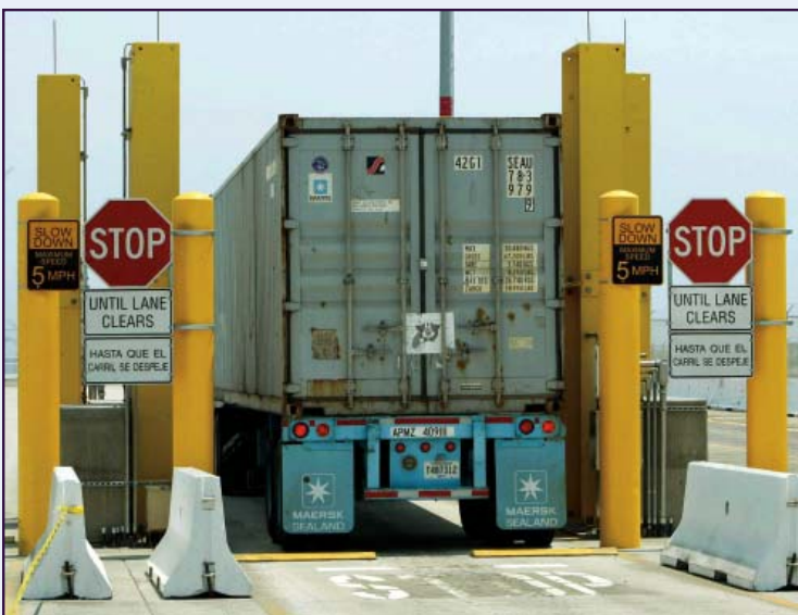
A truck passes through a radiation portal monitor at the Port of Los Angeles, July, 2005.
