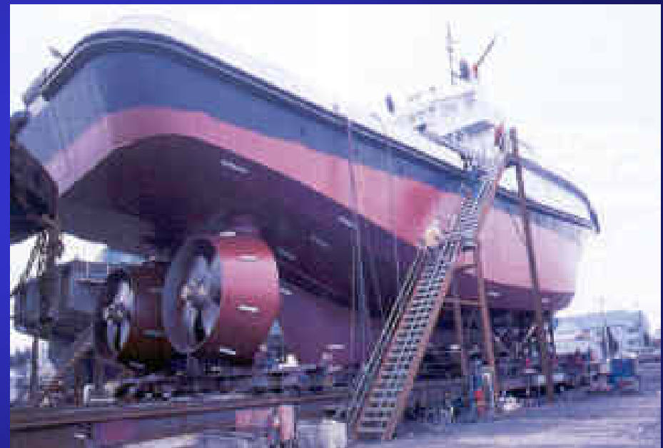
Ulstein-Aquamaster Model US 5001 Z-Drives with controllable pitch
