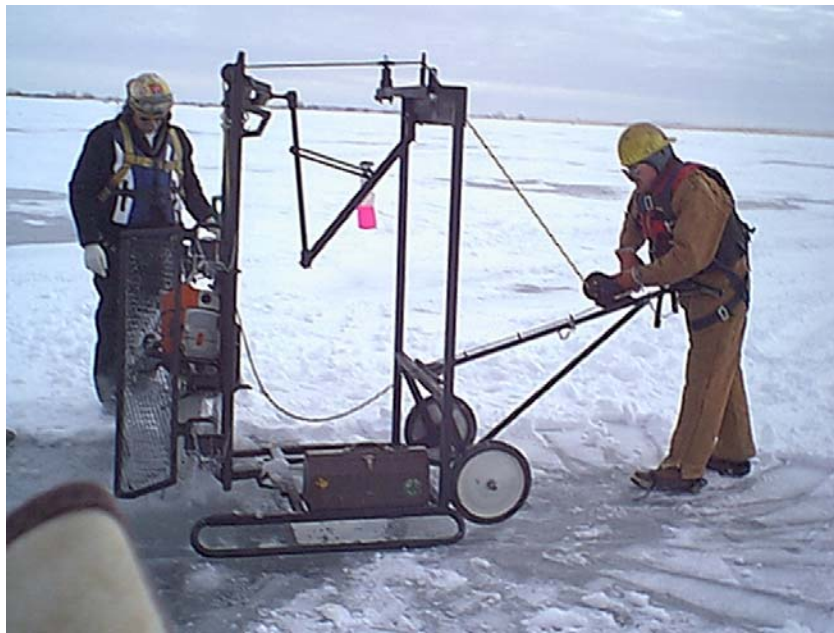
Figure 6. Cutting a slot with the JSG
