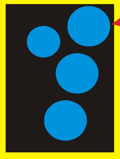
Oil layer is sufficiently viscous to prevent oil droplets from coalescing
