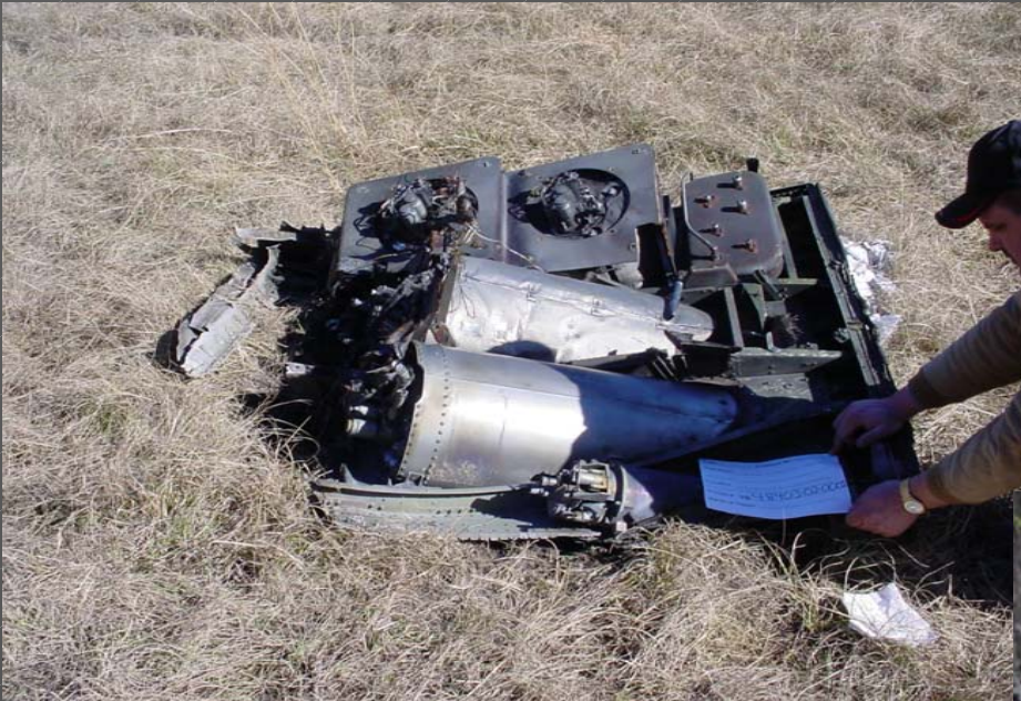
Thruster Structure Assembly
