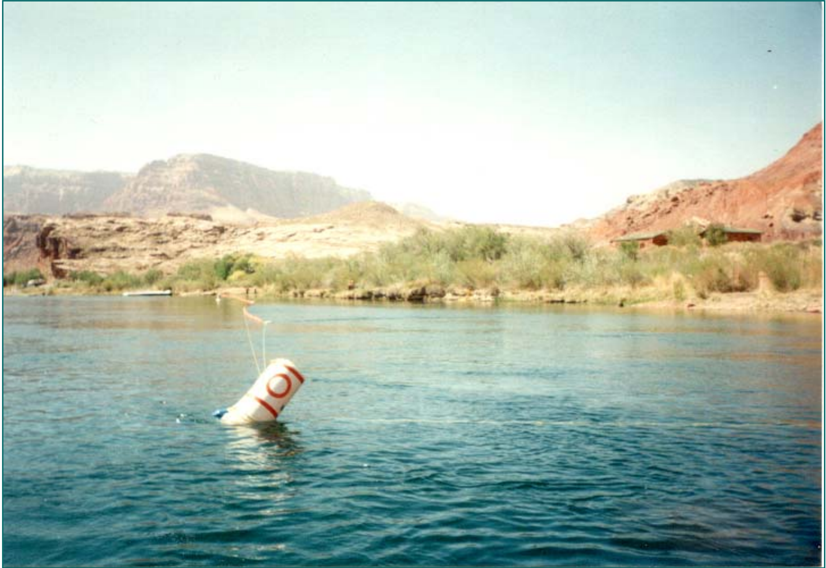
Buoy to Bank Rope Anchor System - Permanent Anchor Placement Colorado River - Arizona
