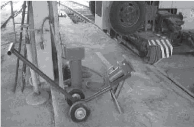
Figure 6. (a) Manual installation of railcar shaker, and (b) cart developed to install railcar shaker without manual lifting.
