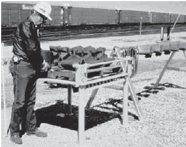
Figure 7(c).. Improved rail yard organization and storage: storage table for coupler knuckles allows lifting at waist height rather than from ground.
