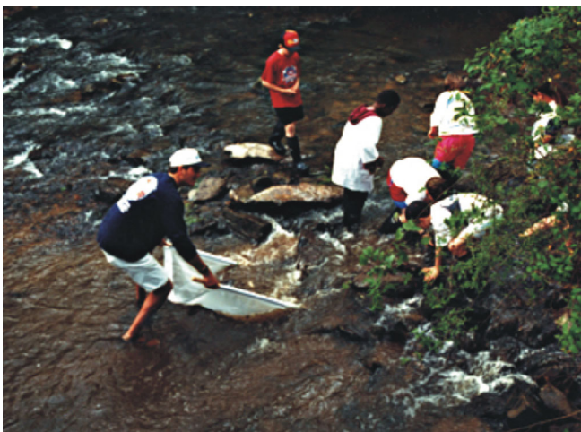
Figure 1: Biological monitoring can be one component of a watershed monitoring program. Information collected on algae, aquatic plants, aquatic insects, and/or fish can be used to assess ecological conditions. The above photo illustrates the use of a kicknet to collect small insects living on the stream bottom. Information such as the types of insects collected, their abundance, and/or the diversity of species provides valuable clues of the health of the stream system.
