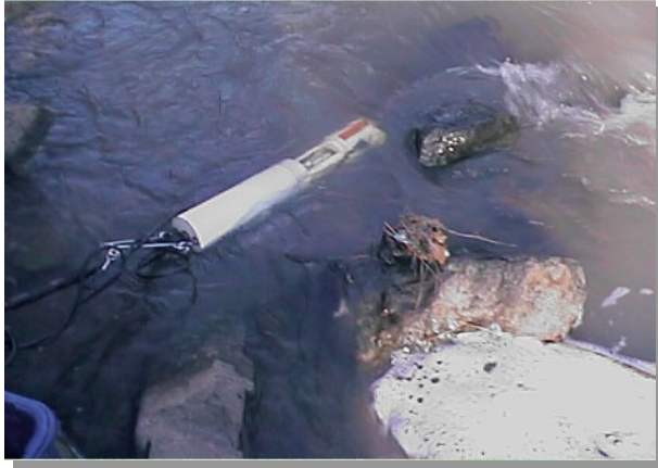
Figure 29: A multi-parameter water quality meter like the one pictured above can collect field measurements such as pH, temperature, conductivity, and dissolved oxygen at the time of sampling.
