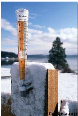
Figure 33: Rain gauges can be as simple as a graduated collection cylinder or as sophisticated as a continuous self-recording device (e.g tipping-bucket rain gauge)
