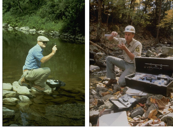
Figure 30: Analytical kits are available for a variety of water chemistry measurements. These monitoring kits are portable, easy to use, relatively inexpensive, and provide practical and quality data. Simple colorimetric comparison kits can be used to measure dissolved oxygen, nitrate, phosphate, chloride, and copper to name just a few of the many analyses.
