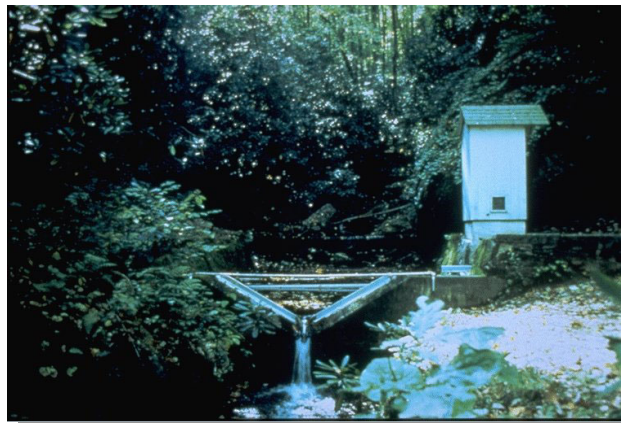
Figure 36: Flow measuring include portable instruments and fixed devices such as weirs and flumes. As illustrated in the above photo, a weir and water level recorder can provide measurements for a wide range of flows.
