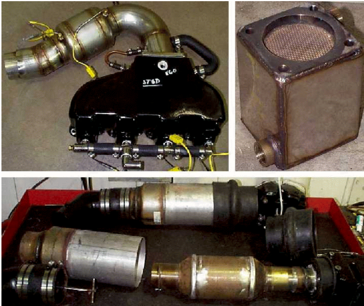
Figure 4.2-1: Three Catalyst Configurations Used in SD/I Test Program
