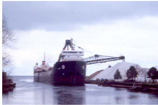
Figure 13. A ship unloads salt at the Thunder Bay River port on Lake Huron. Large vessels enter the river to deliver salt or coal for use by the county and local industry.
