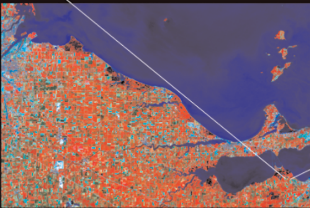
Magnified Image: False-color infra-red PROBE-1 Airborne Sensor Image (August 29, 2001) Scale = 1:3300; Nominal spatial resolution = 5.0 meters
